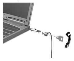
Wrapacomputersecurity lockcable around a nimmovable object such as a table or locked drawer handle. Insert the lock into the notch and turn the key to secure the lock.
